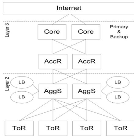
Fig. 3a Partial network architecture of a data center [GJN.2011]
