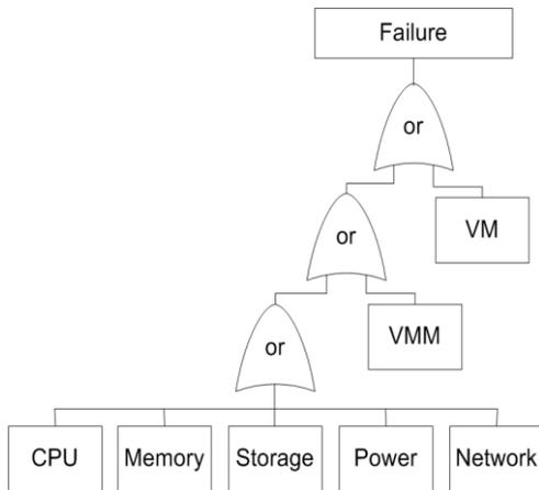
Fig. 2a Fault tree characterizing server failures [JP.2012]
