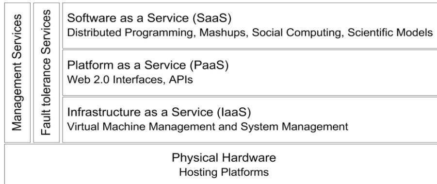
Fig. 1 Layered Architecture of Cloud computing
