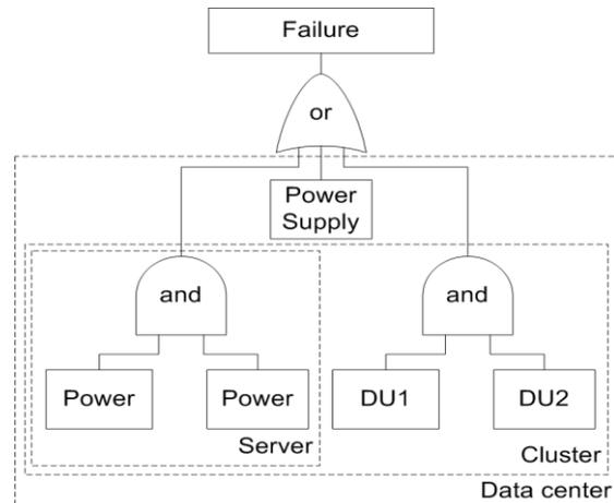
Fig. 2b Fault tree characterizing power failures [JP.2012]
