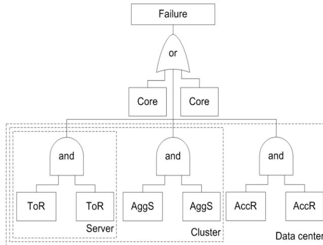
Fig. 3b Fault tree characterizing network failures [JP.2012]
