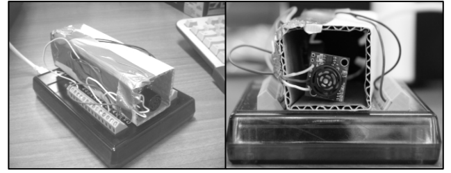
Figure 5: Multi-view image of the experimental device for sensing human presence comprising the distance block and the chemical emission block of Figure 1. The left image illustrates the whole handcrafted device made of a LabJack UE9 (data acquisition unit with Ethernet interface) and a cardboard support for sonar range detection and air quality sensor. In the right image, the sonar range detector is visible in the forefront. A fan (foreground) inside the cardboard jacket is used to convey air towards the air quality sensor (behind sonar range detector).
