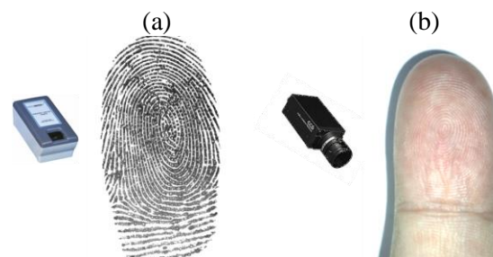
Fig.1. Examples of fingerprint acquisitions performed using different technologies: (a) touch-based image captured with a CrossMatch V300 sensor; (b) touchless image obtained using a Sony XCD-SX90CR digital camera. Touchless fingerprint images present different non-idealities with respect to touch-based images.
