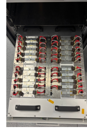
FIGURE 4. Dynamic Gate Stress (DGS) Test-Probe System Device
