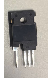
FIGURE 3. SiC Power MOSFET in TO-247 package (SiC Gen3 1200V Power MOSFET delivered by STMicroelectronics)
