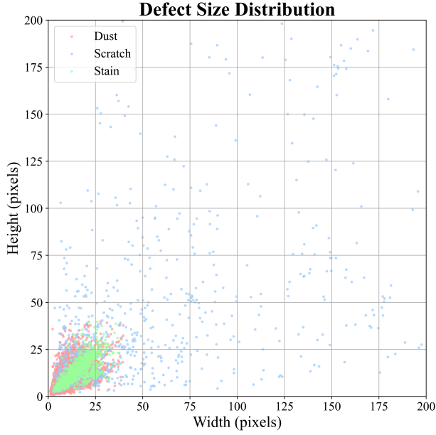
Fig. 7. Empirical Size Distributions of Surface Defects in the PBS-D-RGB Dataset: Dust, Scratch, and Stain Categories with Individually Scaled Axes.
