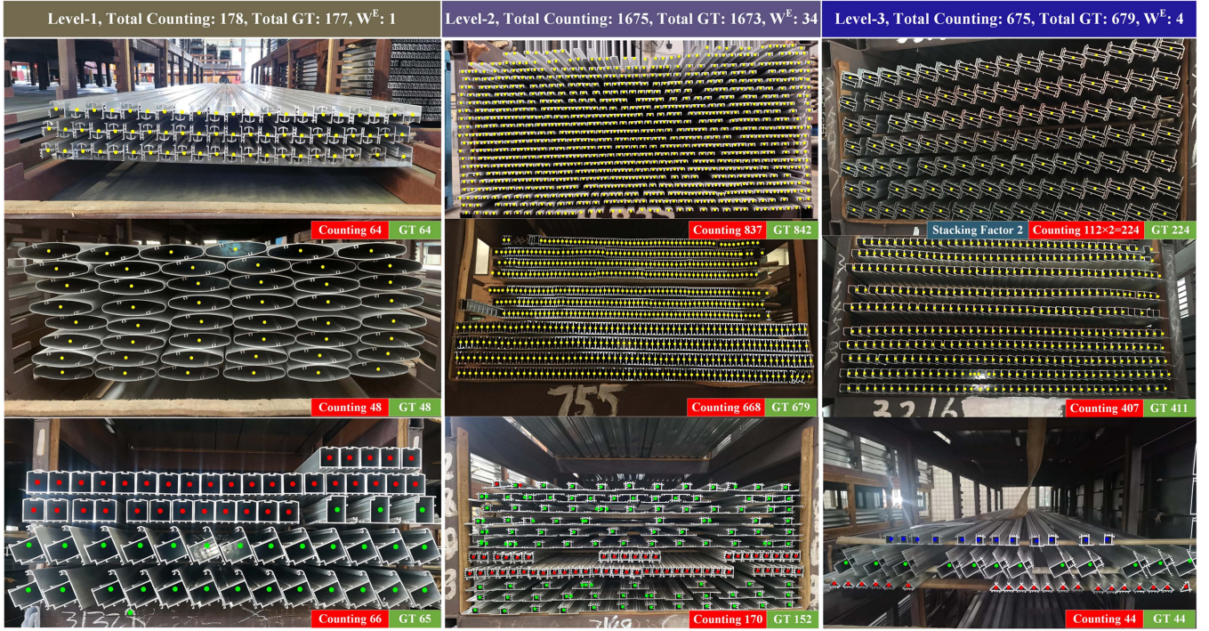
Fig. 5. Proposed method provides visual counting results from Level-1 to Level-3 (the bounding box is replaced by its center point).
