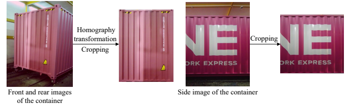
Fig. 4. Homography transformation for the front and rear images of the container and background cropping for the side image.
