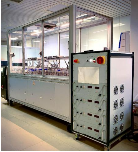
Fig. 5. Power Cycle Test-bench
